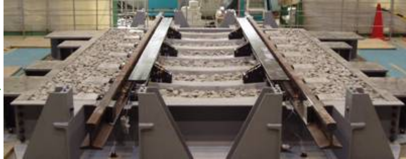
Ballast tracks with Anti-derailing Guard Rails
